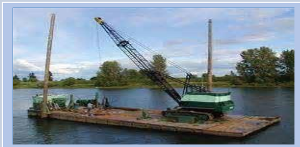
Picture: Barge Mounted Crane (25 T)
