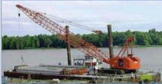
Picture: Barge Mounted Crane (35 T)
